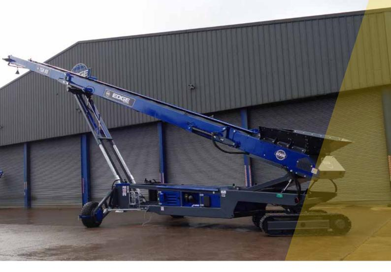
The EDGE TSR80 is a 80ft long tracked mounted conveyor with radial stockpiling functionality. The core design principal for the TSR80 has been to provide customers with an easily transported stacker that can be moved nationally and internationally with minimal fuss or cost. Designed to fit into a 40ft high cube container, with only small assemblies to be refitted upon arrival thanks to its' simple track in, track out philosophy.
